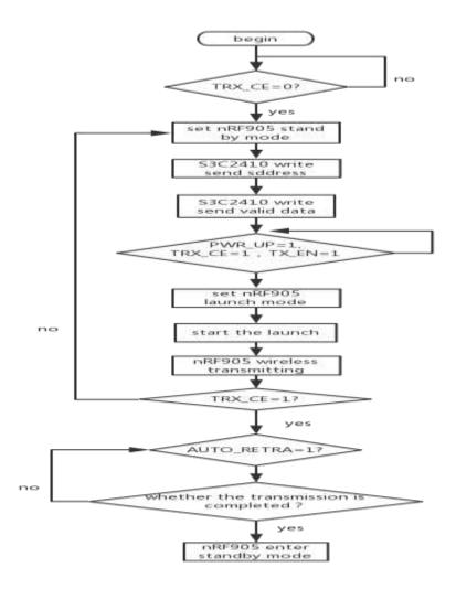
Fig. 5 Wireless transmission flow chart
