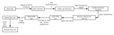
Fig. 1 PKE overall work flow chart II. Keyless Enters The System Overall Design
