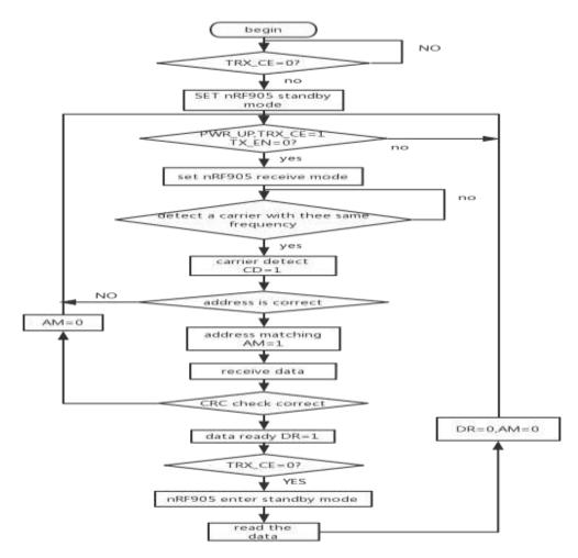
Fig. 6 Wireless receive flow chart
