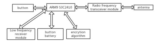
Fig. 2 PKE"key" overall block diagram
