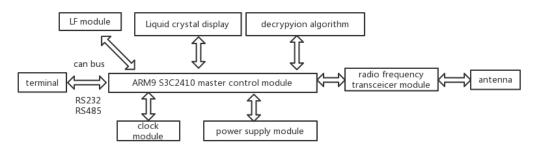
Fig. 3 On-vehicle PKE overall block diagram
