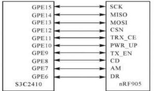
Fig. 4 Diagram of connection between S3C2410 and nRF905
